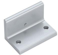
**154 Stabilizer** is a two-piece interlocking set. One piece mounts on the mullion with the top mounting hole 5<sup>3</sup>/<sub>16</sub>" (148mm) below the centerline of the strike; the other piece mounts on the door. Shims are provided to adjust for misalignment between the door and mullion.
